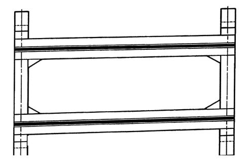
Poor bridge tracking can be caused by any number of reasons. <u>Runway misalignment is the</u> <u>number one cause.</u> However, surveying a runway is extremely expensive compared to checking square of the bridge structure and true parallel alignment of the bridge wheels
