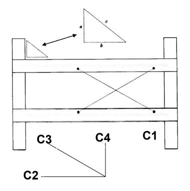
BRIDGE CONSIDERED SQUARE IF WITHIN 3/16" OF MANUFACTURER'S ORIGINAL DIMENSIONS Pythagorean's theorem is <u>one</u> quick method of checking <u>structural</u> square. It is not as accurate nor is it indicative of **TRUE PARALLEL ALIGNMENT**
